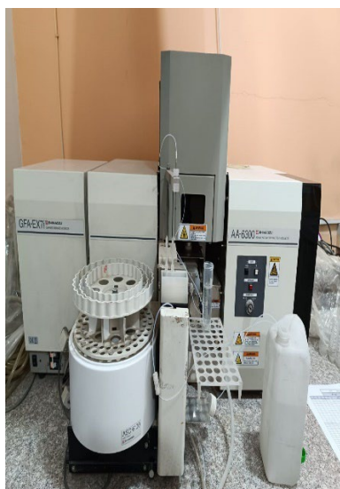
Figure 3 Graphite (furnace) atomic absorption instruments the used in the measurement of the concentrations of elements
