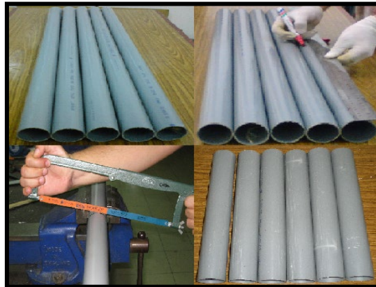
Figure 2. Pipes Cutting and Optimal Pipes for Specimens Fabrication
