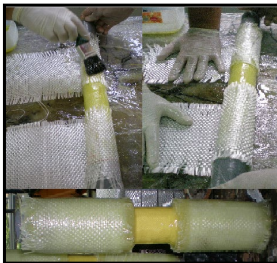
Figure 3. Handle Fabrication of the Specimen (Kevlar Fiber)
