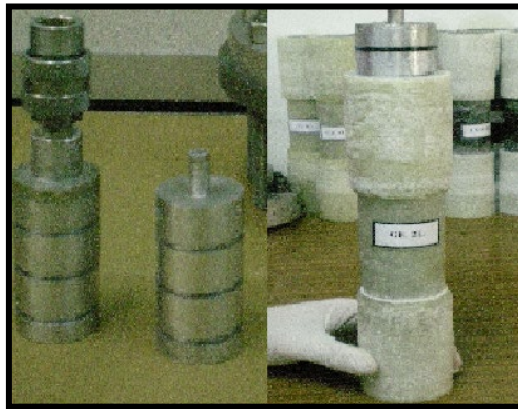
Figure 5: Metal Plug and it is Modification for Testing Procedure (Glass Fiber)
